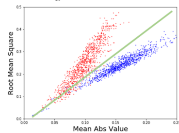
Fig. 3. Extracted data points of EMGs with the linear boundary of our model.
