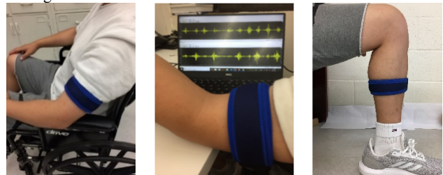
Fig. 2. (Left & Right) An SCI subject wearing our fabric sensor on his upper and lower limb respectively. (Medium) The real-time recording for the EMG signal.
