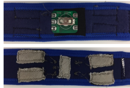
Fig. 1. (Top) Microcontroller integrated into the textile sensor for EMG measurement and wireless transmission. (Bottom) The configuration of our fabric EMGs.
